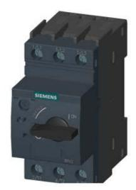
CIRCUIT-BREAKER SZ S0, FOR MOTOR PROTECTION, CLASS 10, A-REL.1.8...2.5A, N-REL.33A SCREW CONNECTION, STANDARD SW. CAPACITY
