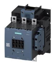
Power contactor, AC-3 185 A, 90 kW / 400 V AC (50-60 Hz) / DC operation 220-240 V UC Auxiliary contacts 2 NO + 2 NC 3-pole, Size S6 Busbar connections Drive: conventional screw terminal
