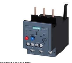
Overload relay 62...73 A Thermal For motor protection Size S2, Class 10A Contactor mounting Main circuit: Screw Auxiliary circuit: Screw Manual-Automatic-Reset
