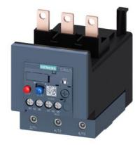
Overload relay 80...100 A Thermal For motor protection Size S3, Class 10 Contactor mounting Main circuit: Screw Auxiliary circuit: Screw Manual-Automatic-Reset
