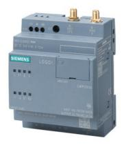
LOGO! CMR2020 communication module for connection LOGO! 8 to GSM/GPRS network; 1 RJ45 port for Ind. Ethernet connection to LOGO! 8; 2xDI; 2xDQ; Write/read access to LOGO! tags; Text message sending/ receipt; E-mail sending; Position detection GPS; Time synchronization/ forwarding with real-time clock; Configuration/diagnostics via web interface; Remote access via OpenVPN/HTTPs, DynDNS; Observe national approval! Manual available as a download
