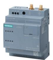
LOGO! CMR2040 communication module for connection LOGO! 8 to LTE network; 1 RJ45 port for Ind. Ethernet connection to LOGO! 8; 2xDI; 2xDQ; Write/read access to LOGO! tags; Text message sending/ receipt; E-mail sending; Position detection GPS; Time synchronization/ forwarding with real-time clock; Configuration/diagnostics via web interface; Remote access via OpenVPN/HTTPs, DynDNS, observe national approval! Manual available as a download
