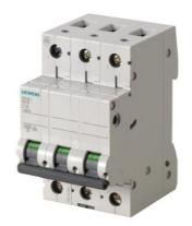
Miniature circuit breaker 400 V 6kA, 3-pole, B, 25A
