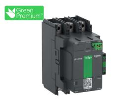
High power contactor, TeSys Giga, 3 pole (3NO), AC-3 <=440V 115A, standard version, 100...250V wide band AC/DC coil
